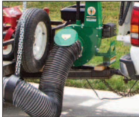
Optional CustomFit™ hanger kit Easy to install, locks in place with 2 bolts. DL1302, DL1402 and DL1802 models only. (Part No. 812260)
