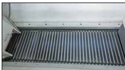
30.25" wide conveyor with 1/2" bars
