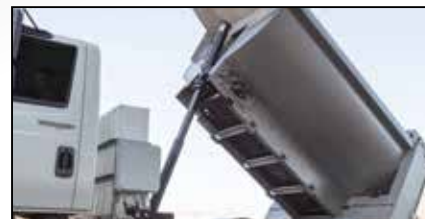
Mailhot® multi-stage, double-acting, nitrided cylinder, trunnion-mounted hoist
