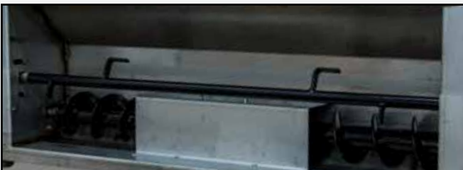
5" Dia. Auger and mixing tines *(5535000)
