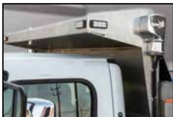
Cab shield with Built-In Tarp System
