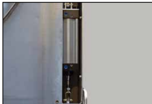
Dual air tailgate cylinders standard
