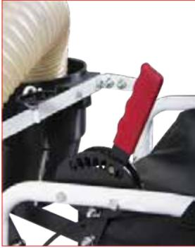
Instant nozzle height adjustment from operator's position, for non-stop, pavement-to-turf leaf and debris clean-up
