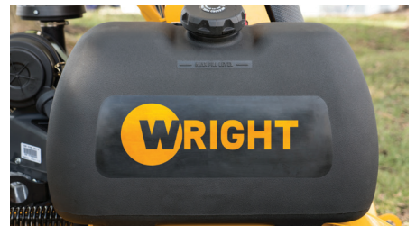
8 Gal fuel tank. Very thick and solid construction is puncture resistant and bolted down to frame. White face fuel gauge is hermetically sealed and magnetically controlled by sender inside tank.
