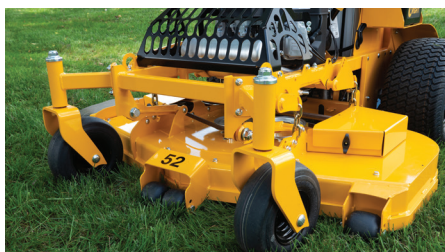
11ga Laminated deck construction with reinforced nose.
