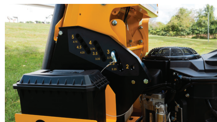
Floating deck and easy to use height selector.
