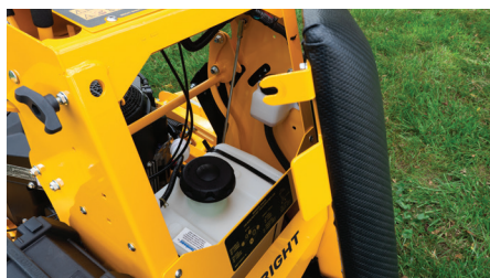
Easy access to service (hinging pad and rear shield).
